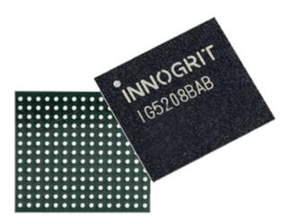
Shasta (IG5208) is an industry-leading PCIe Gen3 x2, NVMe 1.3 SSD controller with capacity up to 2TB.
